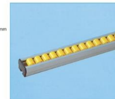
Aluminium slide way SQ-38 Aluminium framework ( W*H): 30mm*22mm Total height( include wheel): 24mm ABS roller : φ13*14mm Roller shaft : 45# Galvanization steel Distance of roller shaft : 15mm,30mm Quantity : 66pcs,23pcs/meter Workload of single roller shaft : 4kg Workload of each meter : 80kg
