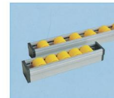
Aluminium slide way SQ-41A Aluminium framework ( W*H): 41mm* 35mm Total height( include wheel): 38.5mm ABS roller : φ28*25mm Roller shaft : 45# Galvanization steel Distance of roller shaft : 30mm,45mm,60mm Quantity : 33pcs , 22pcs , 16pcs/meter Workload of single roller shaft : 10kg Workload of each meter : 100kg
