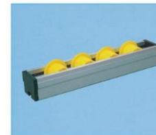
Aluminium slide way SQ-41A Aluminium framework ( W*H): 41mm* 35mm Total height( include wheel): 38.5mm ABS roller : φ38* 28*25mm Roller shaft : 45# Galvanization steel Distance of roller shaft : 45mm , 60mm Quantity : 22pcs,16pcs/meter Workload of single roller shaft : 10kg Workload of each meter : 100kg
